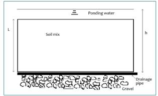
**Figure 9.** Cross section of a rain garden showing the height of water above the drain (h) and the depth of the soil (L) of Darcy's Law.
