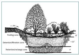
**Figure 8.** Typical cross section of a rain garden. (Source: George's County, Maryland)
